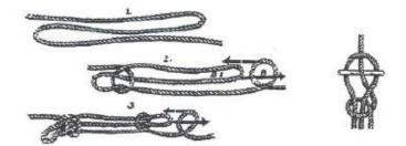
Fisherman's Knot - Useful in tying together anything smooth and stiff, such as nylon fishing wire. It does not slip and is easily untied. Lay the two ropes parallel, then with the end of each tie an overhand knot about the other. Pull the two standing parts.
